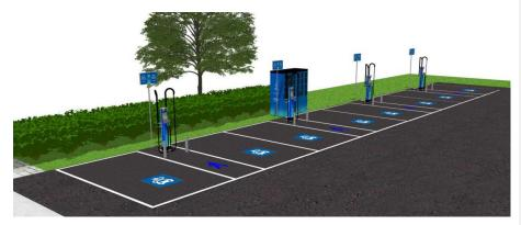
Figure 13: Design for proposed residential charging hub at Chapel Street car park and Quay Road car
